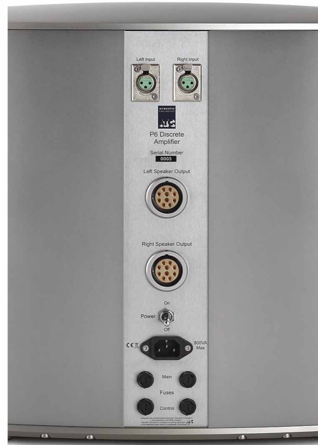
Fig. 6 P6 Connection and Control Panel
